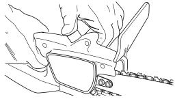
Figure 8 - Pressing Oil Cap to Oil Chain
